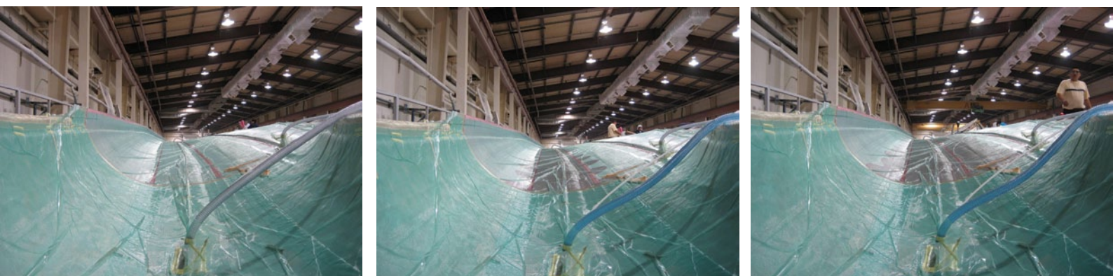
Infusion process using PRIME™ 20LV
